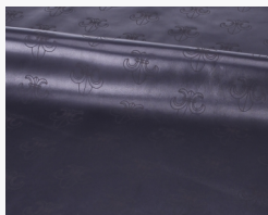
大幅面皮革激光雕花 Leather laser carving
