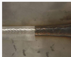
不锈钢激光清洗 Stainless steel laser cleaning
