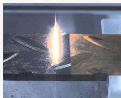
激光清洗锈蚀 Laser cleaning corrosion
