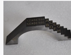
梯形激光打标 Trapezoidal laser marking
