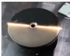
氧化层激光清洗 Laser cleaning of oxide layer
